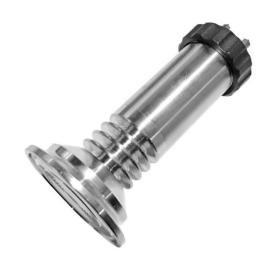
PCM1350 flush pressure transmitter is applicable to food, beverage, pharmaceutical and biological engineering. Full metal flush-mounting isolation diaphragm is directly welded with process connection to ensure the precision connection between process connection and measuring diaphragm. Therefore, no additional sealing gaskets are required, and it ensures there are no measurement dead zones.
