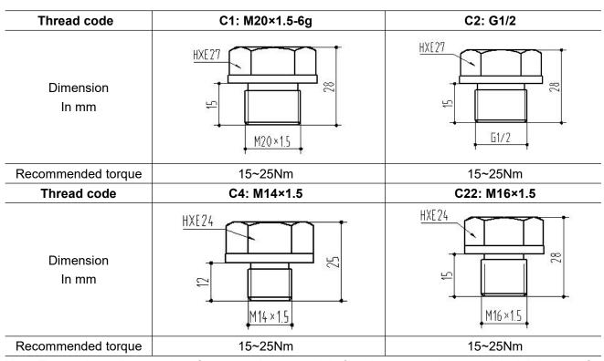
Note: Torque depends on various factors such as material of gasket, supporting materials, lubrication of thread and pressure.
