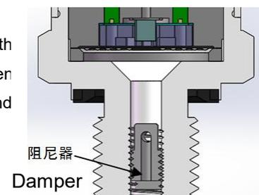
the risk of clogging because the flow of fluid happens in initial start only, the volume of the rear of the nozzle is fixed and the nozzle has a relatively large aperture (1.2 mm).
