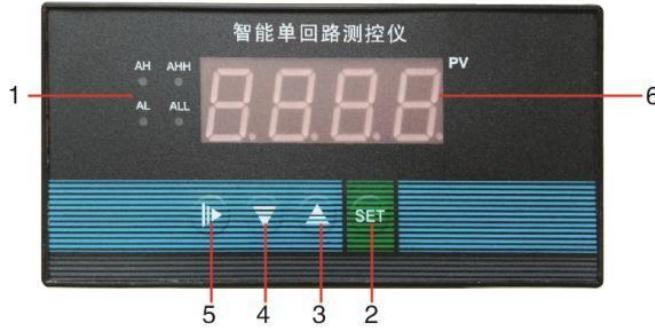
1. Indicator light AH light is on, upper limit relay output; AHH light is on, the top limit relay output;
