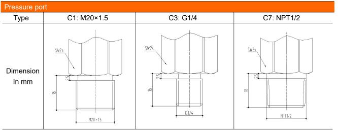
Note: Common threads are M20×1.5, G1/4, G1/2, M14×1.5, NPT1/4 and NPT1/2. Special threads can be customized for batch order.
