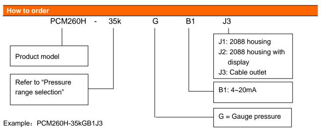
Refer to product model PCM260H, with pressure range  $0\sim3mH_2O$ , pressure reference gauge pressure, output signal  $4\sim20mA$ , electrical connection cable outlet.
