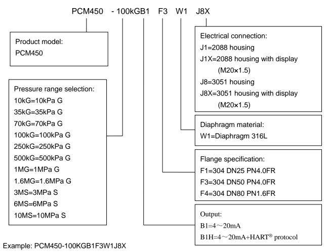
Refer to product modelPCM450, pressure range 100kPa G, output  $4\sim$ 20mA, flange specification 304 DN50 PN4.0FR, diaphragm material 316L, electrical connection 3051 housing with display (M20×1.5).
