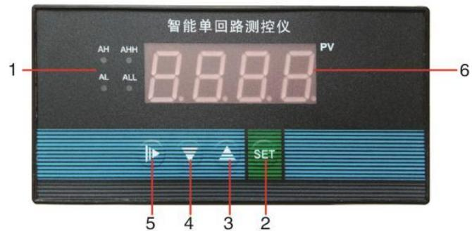
1. Indicator light AH light is on, upper limit relay output; AHH light is on, the top limit relay output; AL light is on, lower limit relay output; The ALL light is on, and the lowest limit relay is output.
