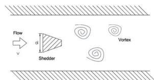
Strouhal Number is a very important coefficient in vortex flow meter, within the range from Reynolds number, Strouhal Number is close to a constant. As showing in the followed chart, St=0.17,vortex shedding frequency is proportional to the flow velocity, from f can be calculated V, the flow range can be calculated by V.
