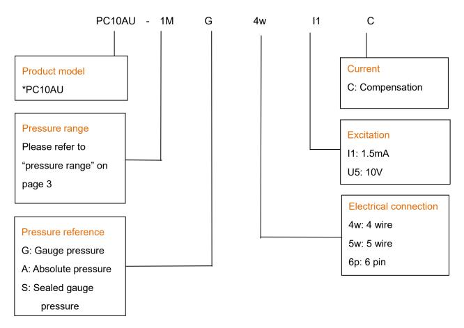
\* PC10AU pressure range <16MPa (Gauge pressure 0.1MPa~4MPa; Sealed gauge pressure 1MPa~16MPa ), please refer to the picture in the section of structure and dimension on the page 3. PC30AU pressure range ≥16MPa (Sealed gauge pressure ≥16MPa), please refer to the picture in the section of structure and dimension on the page 3.
