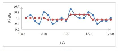
Test data before starting DAP — Test data after starting DAP
