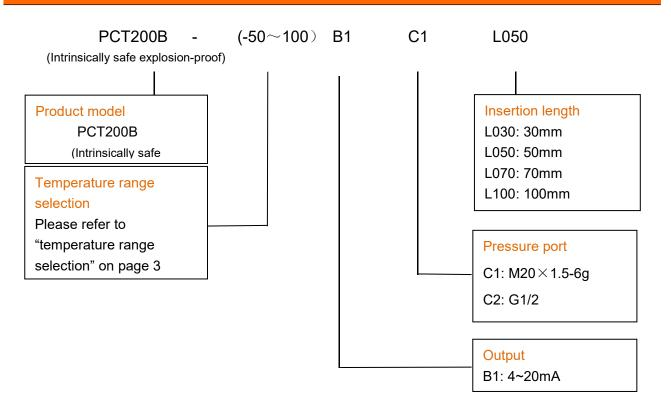
Example: PCT200B (Intrinsically safe explosion-proof) - (-50 $\sim$ 100)B1C1L050 The product model is PCT200B, (-50 $\sim$ 100): temperature range -50 $^{\circ}$ C $\sim$ 150 $^{\circ}$ C, B1: output signal 4 $\sim$ 20mA, C1: pressure port M20×1.5-6g, L050: insertion length 50mm.
