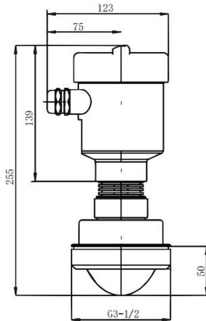
Normal temperature pipe threaded connection
