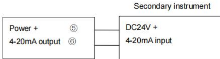
Schematic diagram of the connection of two-wire
