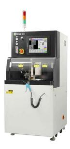
DS830 precision dicing machine uses the DS-300 software control system, imported high-resolution lens and camera to enhance graphics alignment accuracy and efficiency. DS830 is applicable to the cutting process of silicon, PCB, ceramic, glass, lithium niobate, alumina and quartz.
